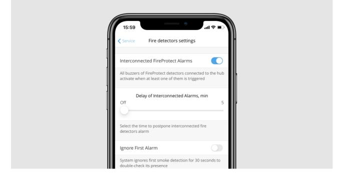
7. If necessary, activate the **Ignore First Alarm** option. This setting is recommended for premises with potential sources of false alarms. For example, if the device is installed in a place where dust or steam can get into the detector.
